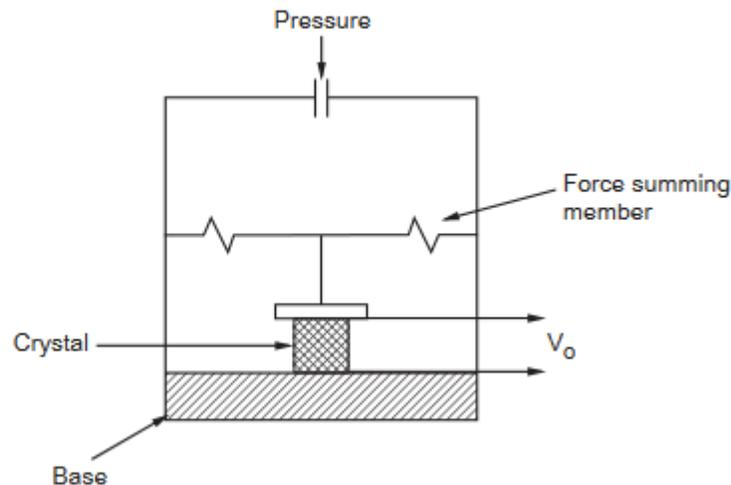
**Fig. Piezoelectric transducer**
