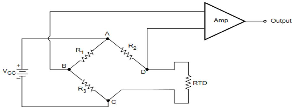
Fig. RTD resistance measurement
