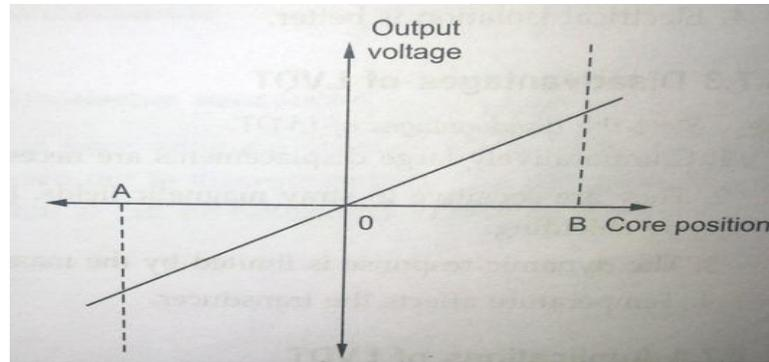
**Fig.** Output Voltage of LVDT at different core position
