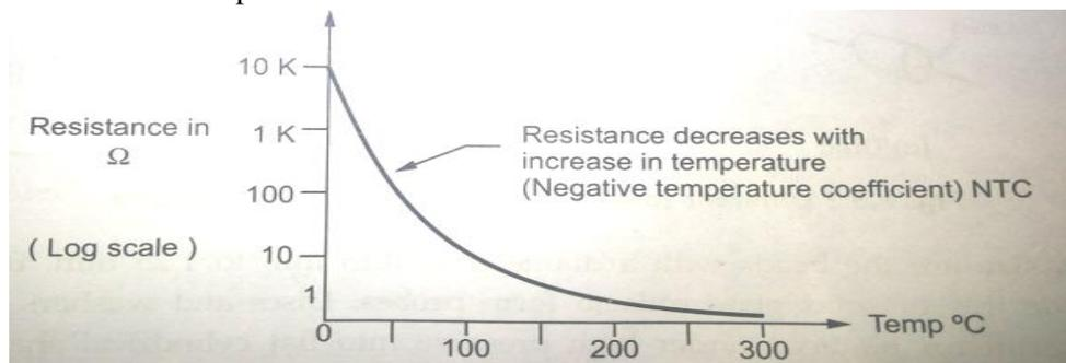
Fig: Resistance versus temperature characteristics of Thermistor.
